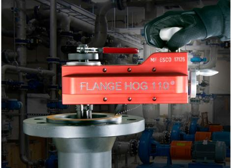
Recondition RF and FF flange gasket seat surfaces with a precise phonograph finish in minutes!
