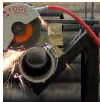
Concrete lined pipe can be cut cleanly. See the Video on our website showing this APS-438LRC with a 12" cut-off blade cutting this 8" concrete lined ductile iron pipe.
