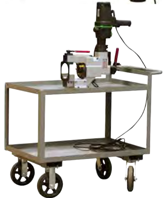
Available cart mount bracket allows complete mobility.
