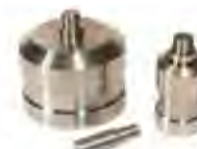
Pilots center the tool and keep it square to the tube. A properly sized pilot is .015" to .030" under the tube I.D. This tolerance ensures smooth operation, long blade life and chatter free bevels.
