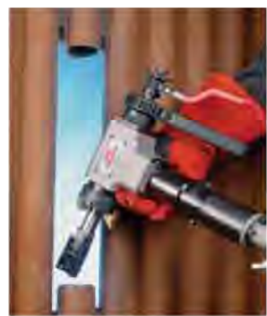
The Wart needs a minimum of 2.625" to fit between tubes in a boiler tube waterwall.
