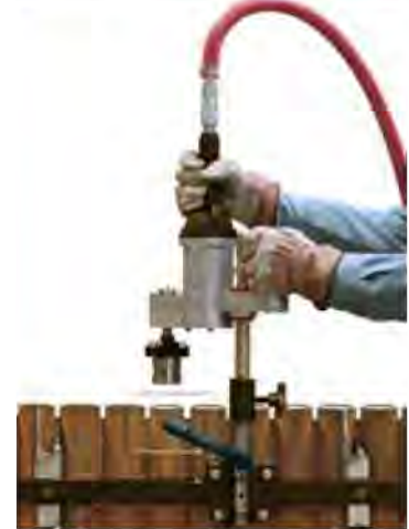
The Track Chassis and Post Assembly's adjustable depth stop ensures all tubes are beveled to the same height.
