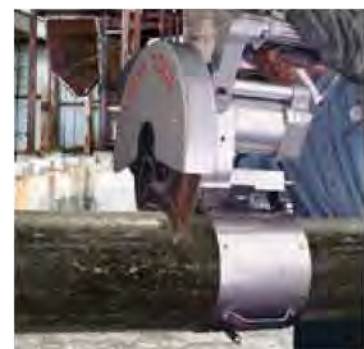
The Escro Wrap Track provides a stable platform for mounting the 3hp air driven saw and produce a clean perfectly square cut.
