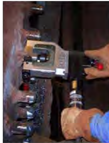
The C-HOG is ideally suited for beveling small bore heavy wall tubes with a high percentage of chrome, stainless steel and other hard alloys.
