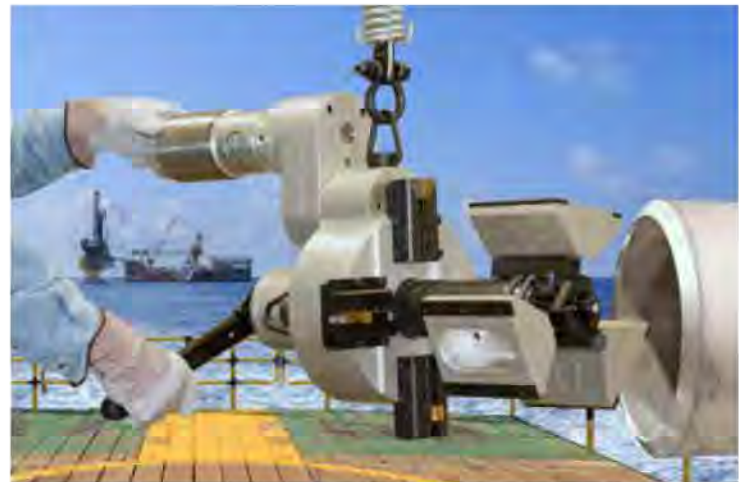
The clamping system of the Commander MILLHOG® Model C-314 pipe beveling machine has six contact points that minimize vibration for chatter free bevels on both thin and heavy wall pipe.
