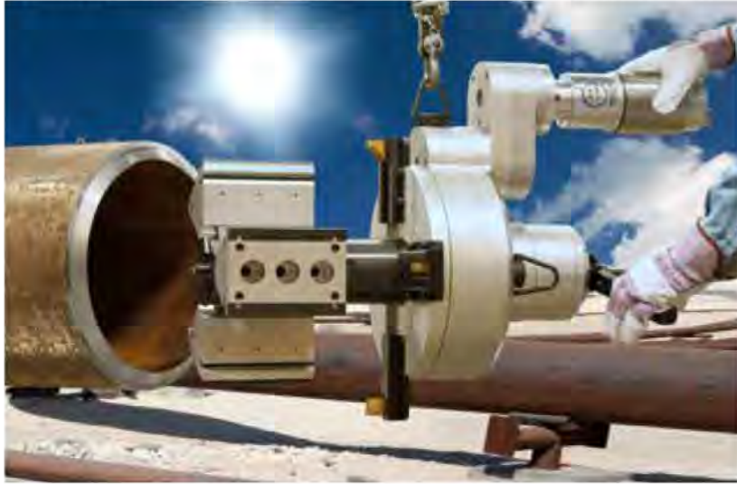
The Dictator can bevel, face and bore heavy wall pipe at any angle at the same time quickly and accurately for perfect fit-up and precision welding.
