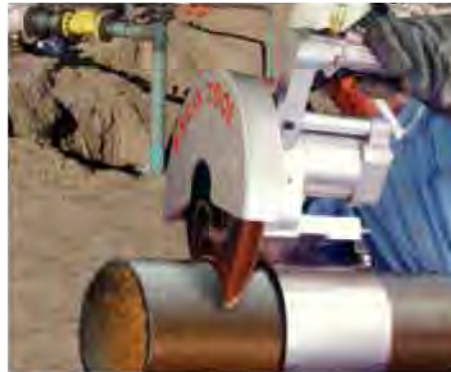
APS-438 cuts 8.0” pipe cleanly and square with no “HAZ” and has a cutting depth of 4.0” (101.6 mm) using a 12.0” Cut-Off Blade.
