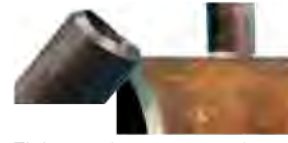
Fish mouth contours tube to fit evenly on header radius.
