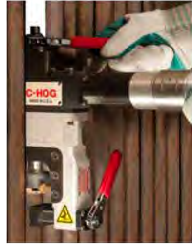
This rugged tool has a narrow profile and can fit between 1.25" O.D. membrane water wall boiler tubes to bevel a single tube for a Dutchmen tube repair.
