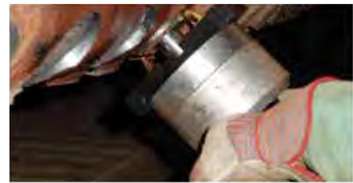
Portable, for on-site and tube beveling. Tube stub weld removal from header also prepares the header for new tube installation.
