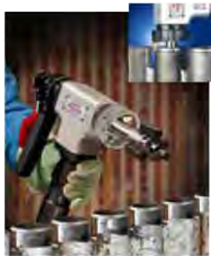
Tube overlay is efficiently removed from the O.D. and the end is simultaneously beveled.
