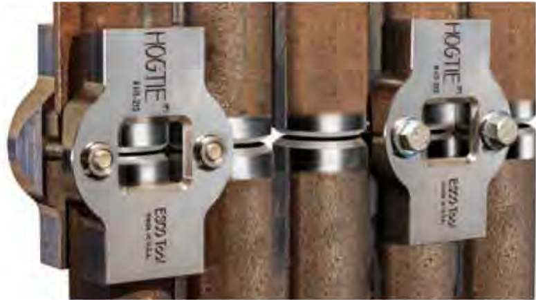
HOG TIE® tube alignment tools speed waterwall boiler tube fit-up and helps reduce tube joint failure due to misalignment.
