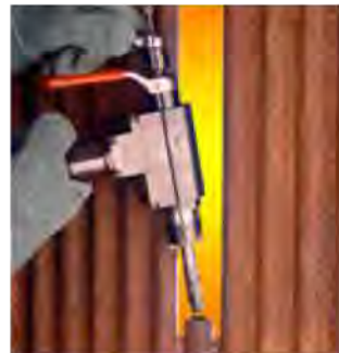
Only 1.5" wide for single boiler tube beveling
