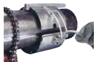
Mount the Wrap Track to the pipe
