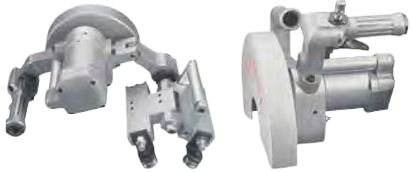
The APS-LRC requires 6.0” (152.4 mm) clearance with Cut-Off blade plunged into pipe and has a cutting depth of 2.0” (50.8 mm).
