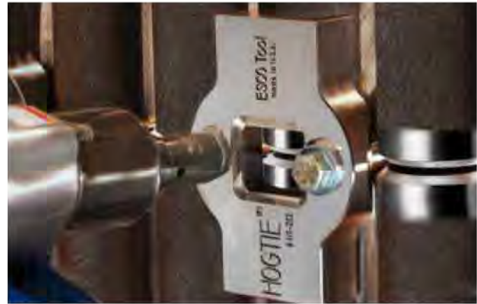
Available impact wrench draws the HOG TIE® assembly together for fast tube end alignment.
