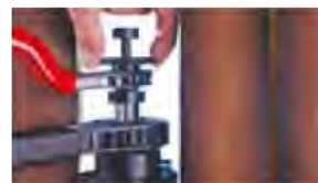
Tube overlay is efficiently removed from the tube O.D. and the tube end simultaneously beveled in preparation for welding.
