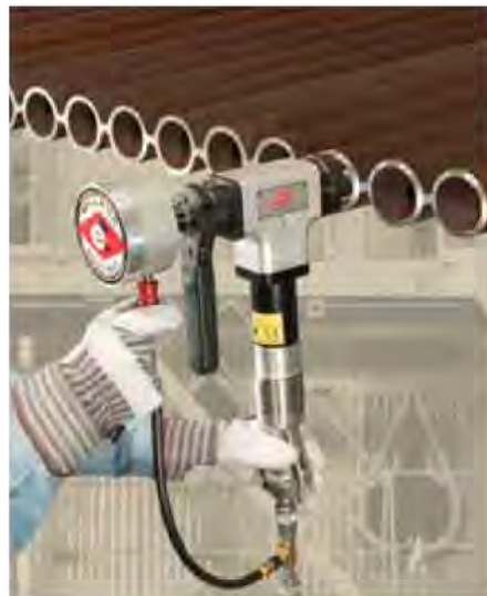
The Air Clamp instantly clamps and releases the tool to the tube and pipe I.D. which saves a time by reducing the cycle time between tube bevels.
